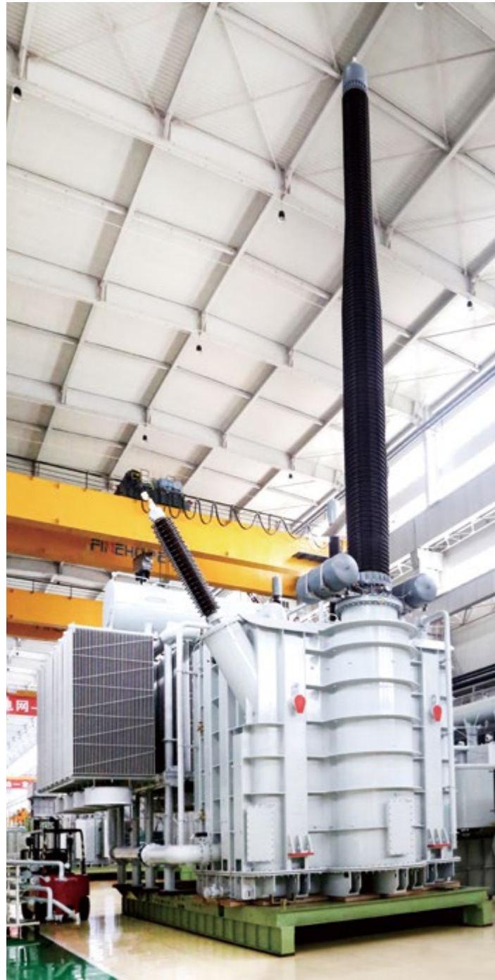
▲ 400MVA/1100kV UHV Shunt Reactor is currently the largest capacity shunt reactor in the world.
